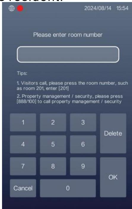
b) When used for a community gate, enter the full 10-digit code to call the resident. For example, input "0101010204". The first 6 digits represent Zone 01, Building 01, Unit 01, while the last 4 digits indicate the room number. Here, 02 means Floor 02, and 04 means Room 04.
