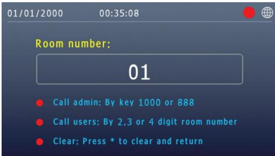
②When used for a community gate, press the entire 10-digit code to call the resident. For example, the first 6 digits represent Zone 01, Building 01, Unit 01, while the last 4 digits indicate the room number. For instance, 02 means Floor 02, and 04 means Room 04.
