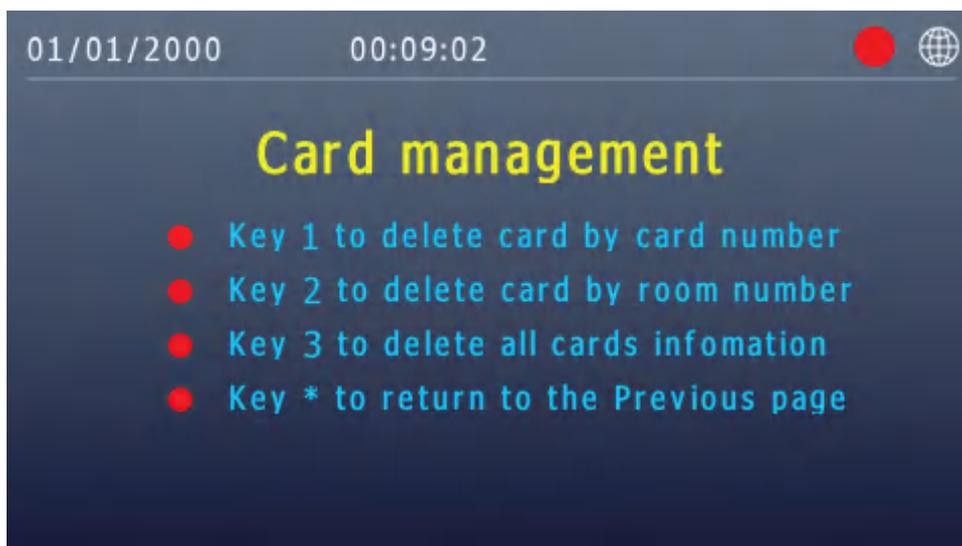
① Press "1" to delete a card by card number. Input the card number or swipe the card, then press "#" to confirm and delete.
