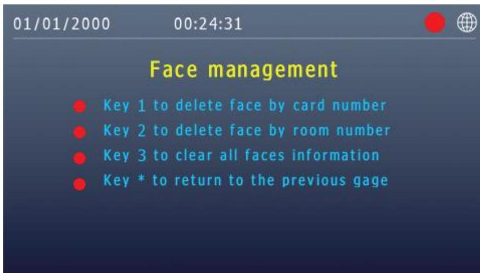
① Press “1” to delete by card number. Swipe the card to retrieve the card number or input it manually. Then press “#” to confirm, or press “\*” to cancel.
