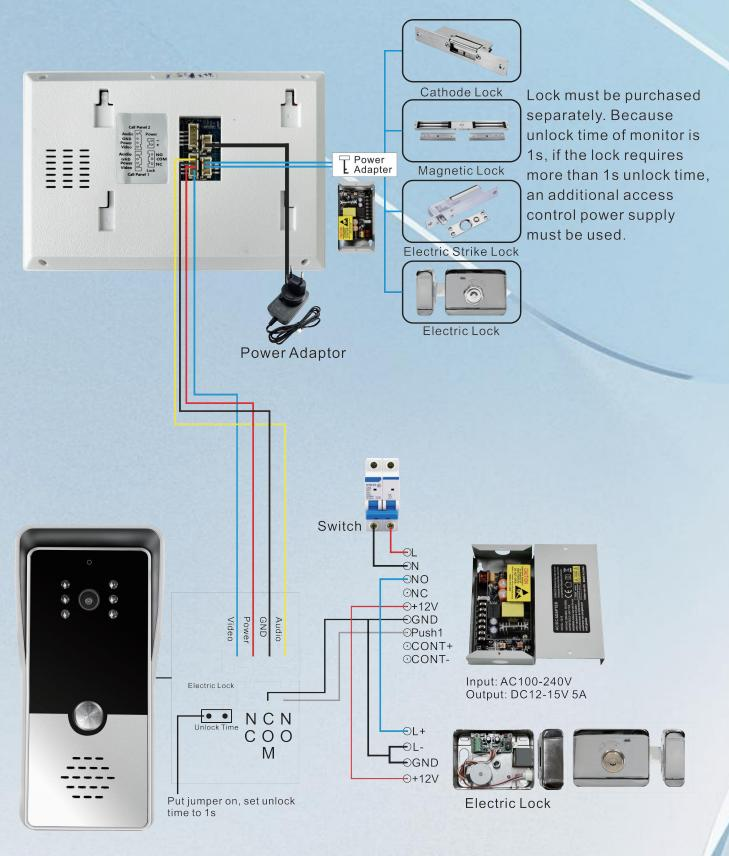
1 Ostation + 1 Indoor Monitor: Connected Directly Through Power Adapter Indoor Monitor Supply Power To Outdoor Station.
